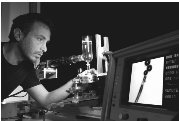
FIGURE 1.6 High-speed video camera used to visualize bubble nucleation sites in a glass poured with champagne (photograph by Hubert Raguet).
